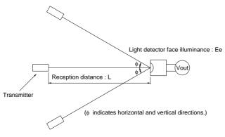
Fig. 2 Standard optical system
