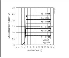
Figure 5a. MAX649 Current-Sense Resistor Graph
