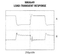
A: LOAD CURRENT (100mA & 1A), 500mA/div B: 5V OUTPUT VOLTAGE, AC COUPLED, 50mV/div
