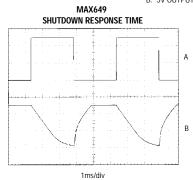
I<sub>LOAD</sub> = 1A A: SHDN INPUT VOLTAGE (0V & 5V), 2V/div B: 5V OUTPUT VOLTAGE, 2V/div
