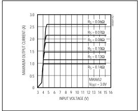
Figure 5c. MAX652 Current-Sense Resistor Graph
