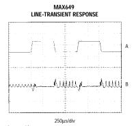
I<sub>LOAD</sub> = 1A A: INPUT VOLTAGE (7V & 12V), 5V/div B: 5V OUT, AC COUPLED, 100mV/div
