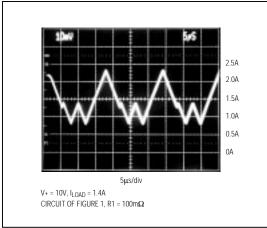
Figure 3b. MAX649 Light/Medium Load-Current Waveform (500mA/div)
