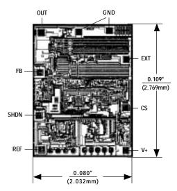
TRANSISTOR COUNT: 442; SUBSTRATE CONNECTED TO V+.
