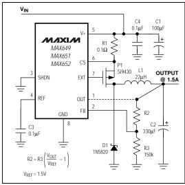
Figure 4. Adjustable-Output Operation
