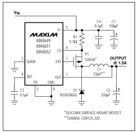
Figure 1. Test Circuit
