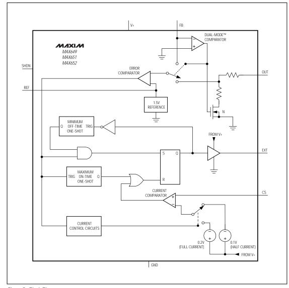
Figure 2. Block Diagram
