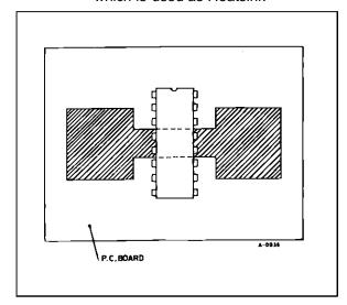
temperaturemust not exceed 260°C and the soldering time must not be longer then 12s. The external heatsink or printed circuit copper area must be connected to electrical ground.
