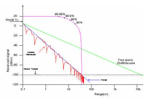
curve for a 433MHz 10mW TX (unity gain antenna)
